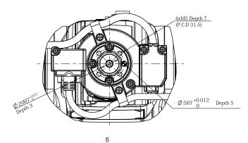
Detailed drawing of base mounting face
