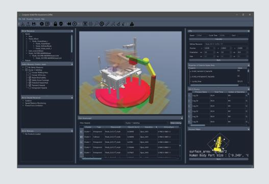
Utilize the CARA\* simulation software to identify risks caused by the robot colliding or getting caught
